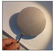
fabrication process is implemented on 4-inch Silicon on Insulator (SOI) technology. A sensor chip size of 2x2.5 mm<sup>2</sup> ensures a yield for wafers exceeding 1000. Present HST production capabilities reach 20,000 sensors per year, with plans to scale up to 200,000 within the next three years.
